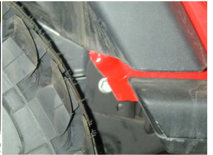
Above – Fender trimmed, vehicle on level ground - 4.5 lift kit, 37x13.5 Toyo's
