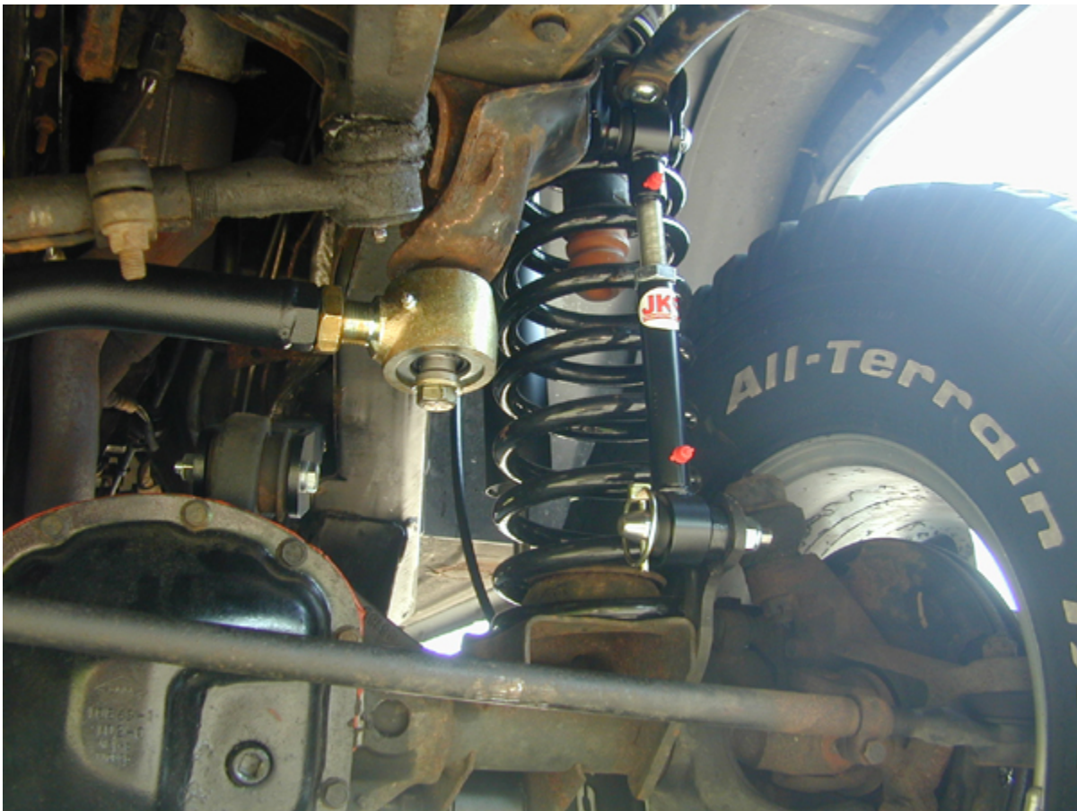
Shown above is a XJ 4.5 inch Clayton Off Road short arm lift with our adjustable trackbar.
