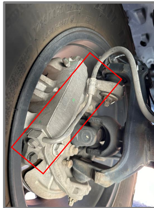
Standard single-piston brake caliper Use 1309101
