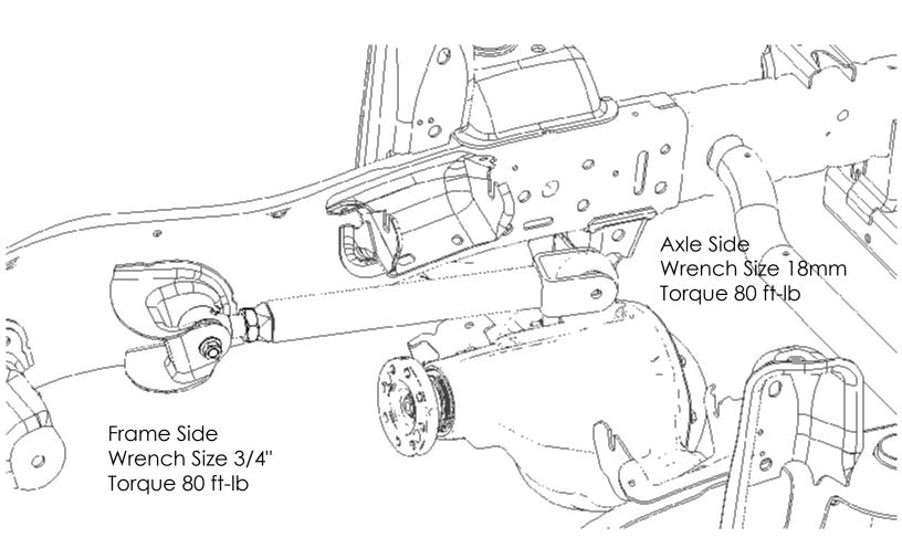
Refer to drawing below for minimum and maximum lengths.
