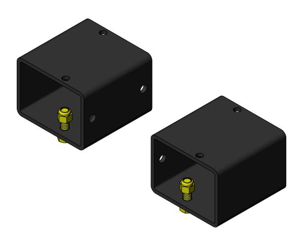
Step 1: For a 3" bump stop locate the tube on axle mount with holes offset to the inside.
