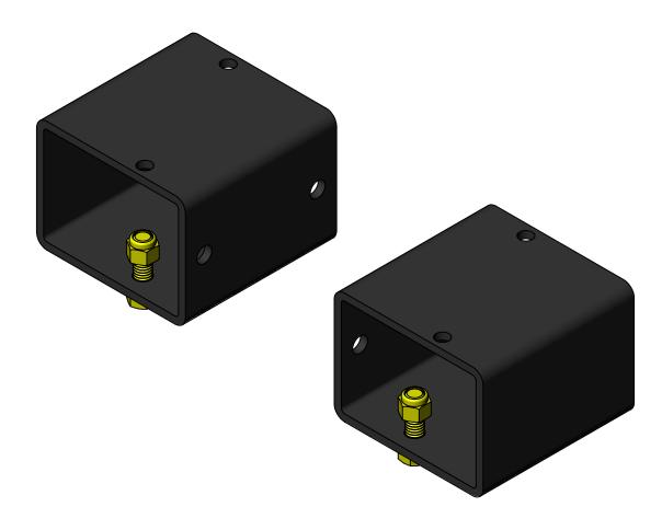
Step 1: For a 3" bump stop locate the tube on axle mount with holes offset to the inside. For a 4" bump stop stand the tube on end. Bump stops will be offset to the driver side. Step 2: Insert bolts from the bottom, thread nuts on.
