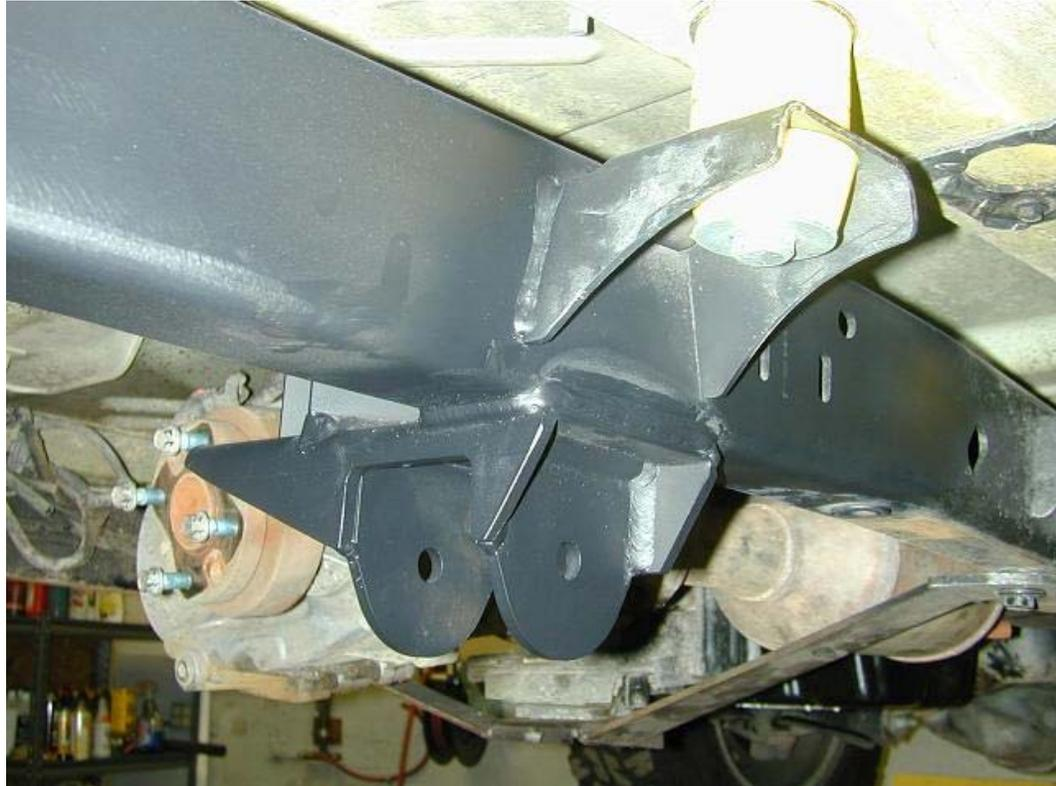
6. Remove clamps and weld all four sides.
