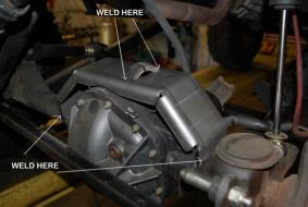
31.32. Welding to both sides of the tubes, and the upper mount gives it superior strength. You can cut the top of the mount off after welding for a clean look, or leave the top mount sticking up. It should not be in the way for the 3 link mount.
