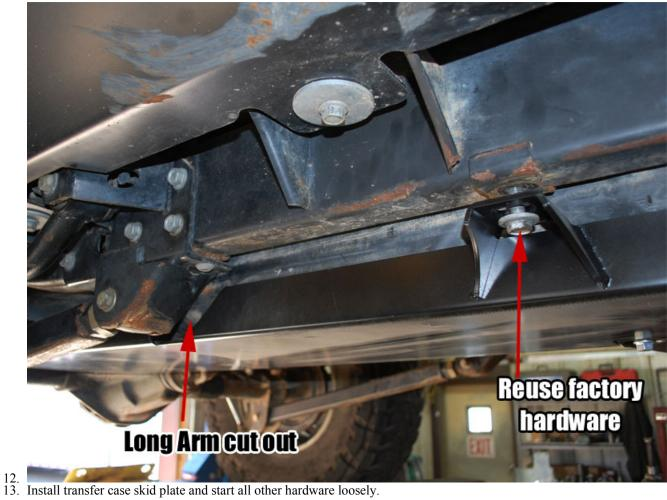
14. Use supplied ½ bolt, washer and lock nut to connect transfer case and gas tank skid plates together. Leave loose at this time!
