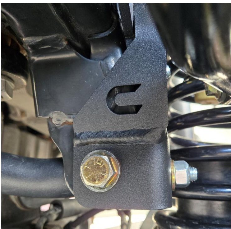
Figure 8: Torqued track bar bolt
