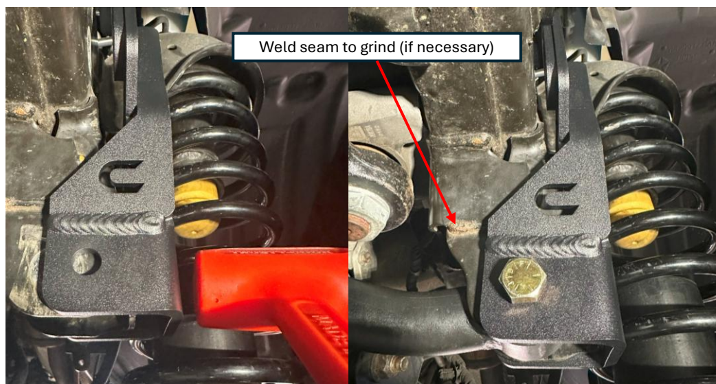
Figure 3: Track Bar Brace with track bar and bolt temporarily installed
