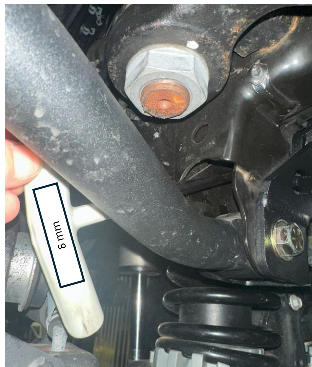
Figure 9: Tightening the remaining hex cap screw
