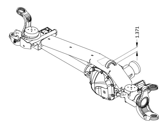
Step 8: Make 5 1" welds along gusset to axle tube on both sides. Step 9: Make 5 1" welds along top of gusset on both sides.
