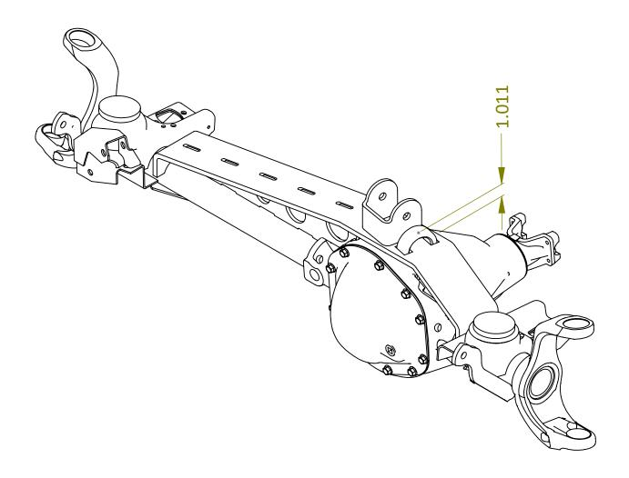
Step 8: Make 5 1" welds along gusset to axle tube on both sides.
