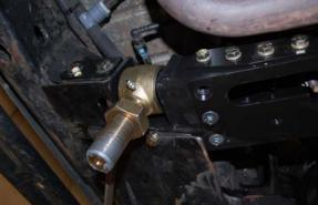
15. This pocket design allows for maximum clearance, however lining up the washers, and bolt is a little tricky. Installing just the johnny joint makes it easier to hold everything in place while you line up the washer, bolt, and nut on the other side. Once everything is installed, an open ended wrench will fit on the outside to hold the nut. On the inside a 13/16 - 3/8 drive socket
