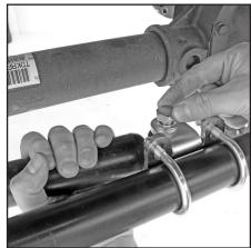
8) Reinstall the end of the factory shock into the bracket. To adjust the shock properly. turn the wheels all the way to the right to the lock and hold them there. Completely compress the stabilizer shock, pull it back out 1/8" and then clamp it down onto the tie rod. Torque the u-bolt nuts to 25 ft. lbs.
