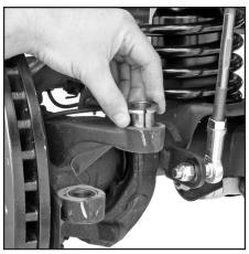
2) In reversed drag link applications only, insert the tapered sleeve into the 7/8" hole.
