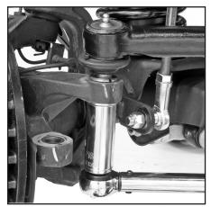
4) Install the supplied nuts at both ends of the drag link and torque to 80 ft. lbs.
