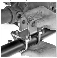
7) Assemble the supplied steering stablizer kit onto the tie rod as shown.
