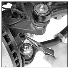
10) Install cotter pins on all foucr tie rod ends.
