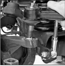
3) In either drag link application, insert the new drag link end into pitman arm and then into the steering arm from either the top or the bottom depending on which kit you are installing.
