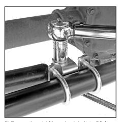
9) Torque the stabilizer shock bolt to 50 ft. lbs.
