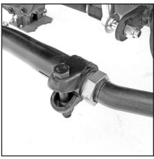
12) An alignment shop can use the double adjuster at the driver's side of the tie rod and the pitman arm end of the drag link to center your steering wheel and realign your steering.
