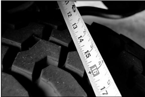
**HINT:** For example, measure from the edge of a tire tread lug to the outboard side of chassis, then repeat the measurement on other side of vehicle using exact same points.
