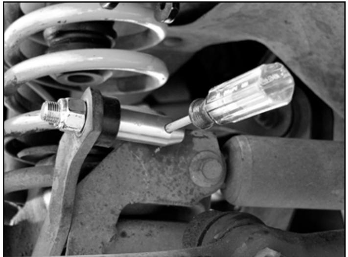
**HINT:** A small Philips head screwdriver or punch inserted into the Click Pin hole will enable you to prevent the mounting post from rotating when tightening the nut.
