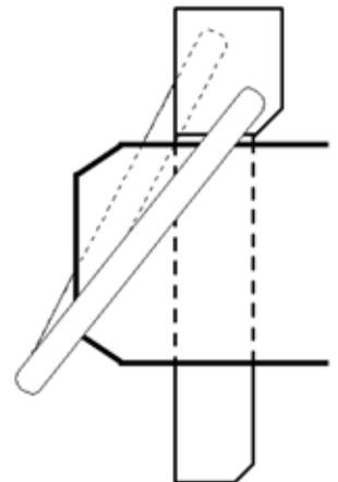
*When properly installed, the ring on the Click Pin will "snap" against the shaft of pin. When installed backwards, the ring does not fit snugly against shaft.*
