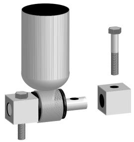
O Slide remaining Mounting Block (B) onto opposite end of Cross Pin (A).
