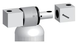
IMPORTANT: This product is designed to preload the shock absorber bushings for maximum performance and longevity. Therefore, you should find it necessary to compress the bushing approximately 1/16" to 1/8" before the mounting bolts and/or roll pins can be inserted.
