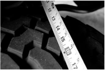
**HINT:** For example, measure from the edge of a tire tread lug to the outboard side of the chassis, then repeat the measurement on the other side of vehicle using the exact same points.
