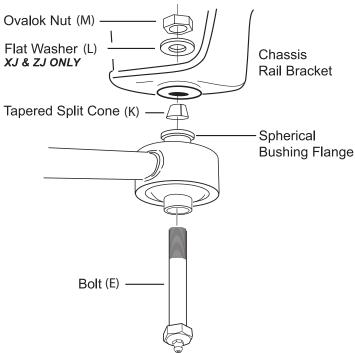
**HINT:** Tapered Split Cone (K) should be located between flange of spherical bushing (G) and mounting surface of chassis rail bracket, with the narrow end of tapered cone facing up towards chassis.
