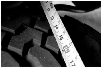
O If the two measurements are equal, the axle is centered. If the measurements vary, divide the difference in half to determine the amount of adjustment required. HINT: If the axle housing is not centered, the chassis can be laterally shifted using either of the following methods.
