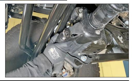
With a 15mm wrench or socket, remove all of the bolts that attach the factory steering stabilizer shock axle bracket to the axle, and remove and discard the bracket.
