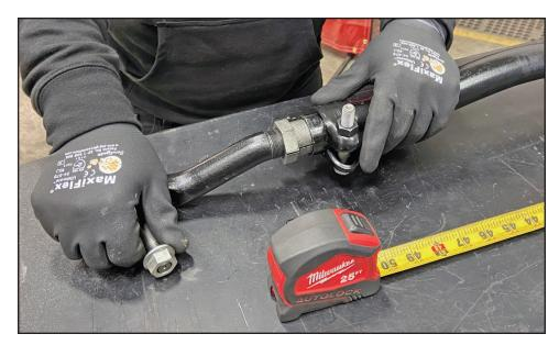
See the guide below for tie rod adjustment measurements. Pre-adjust the passenger's side of the tie rod to the dimensions illustrated below (RH side shown below) before installing the unit into the vehicle. After installation, do the rest of your adjustments with the double adjuster on the driver's side.
