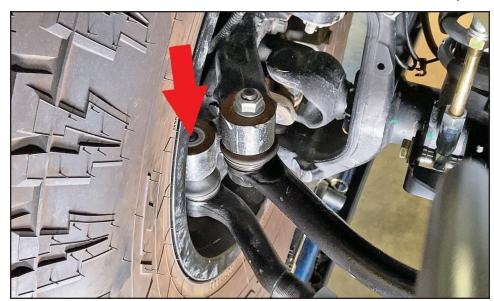
Step 23 Next, insert the new tie rod at the passenger's side knuckle....
