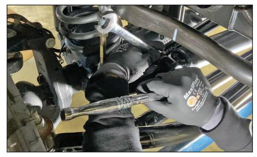
Now we'll move on to removing the stock tie rod from the passenger's side knuckle. Remove the tie rod end attaching nut with a 21mm wrench and a 10mm wrench on the stem of the rod end.
