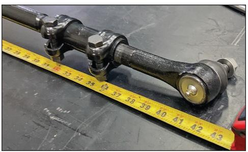
Adjust your new drag link's center to center dimension per the Tech Tip below. Loosen the adjuster hardware with an 18mm and a 19mm wrench if necessary.
