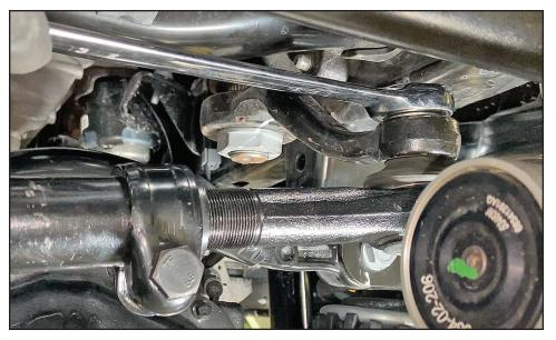
Step 27 Install a cotter pin thru the hole in all 4 tie rod ends and bend over with your needle nose pliers.
